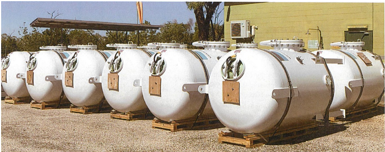
Small carbon steel pressure vessels that were delivered in April
